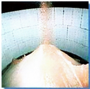
UHMW-PE Lined storage silo
