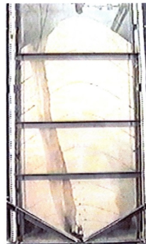
Problems with flow in animal feed storage bin
