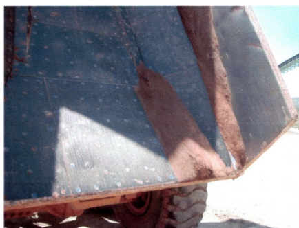
figure 3.1.4d – Abuse from excavator operator
