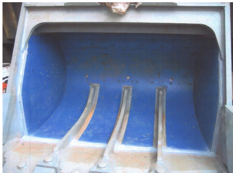
A complete stud weld installation on an excavator bucket.
